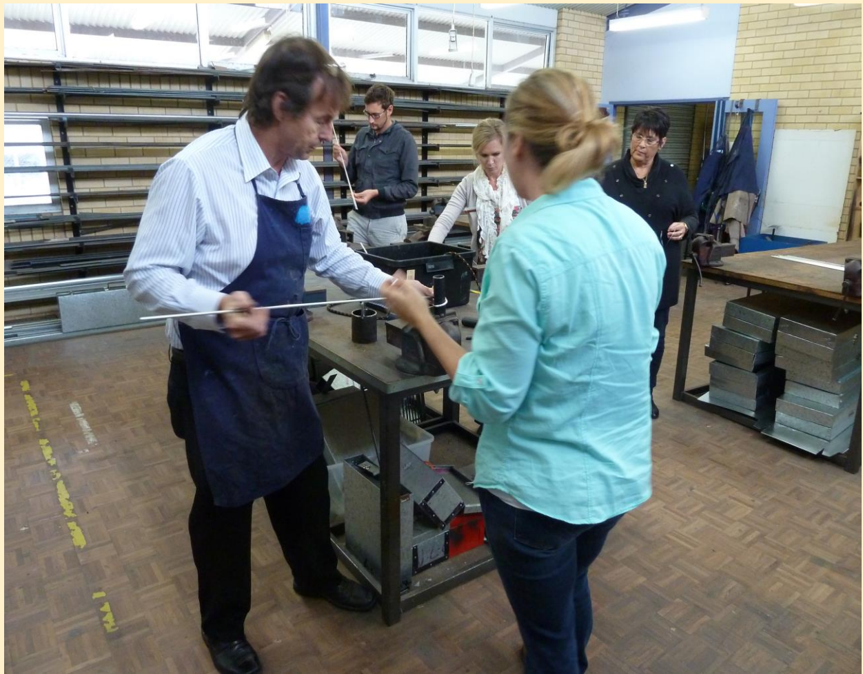
Fig. 6 Andrew Burgess demonstrating the use of a jig to successfully bend the aluminium rod
